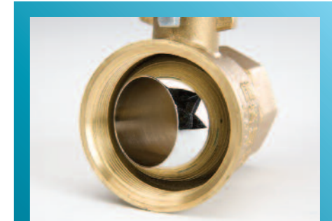
Ball is DZR brass chrome plated, designed for a long life. Ideal for chilled water applications. Temperature range is -10 to 120°C. Ball is full bore.
